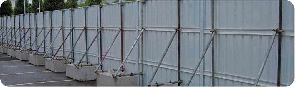
Safe Hoard™ is a 2.4m steel on-ground site hoarding, secured by our 750kg concrete or, NEW ultra-low carbon (ULCC) blocks. As an on-ground site hoarding, Safe Hoard™ requires no ground excavation and no risk of potential service strikes which may
