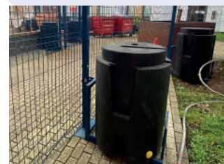
Water Filled Ballast
