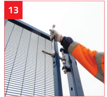
13 Adjust all Hinges to bring Gate Leafs into position.
